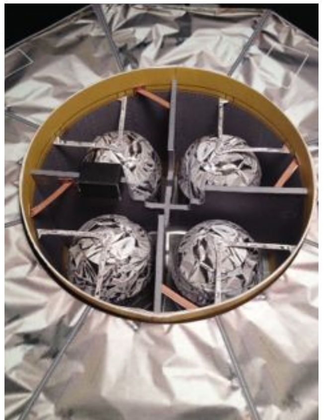
Back side of Top Debris Panel. Each MMS Observatory will have a unique Orbital Debris Panel with its corresponding color (Gold, Blue, Green or Purple)
