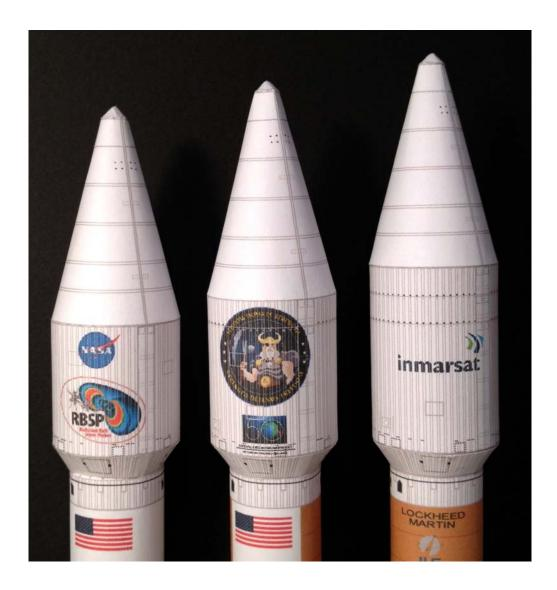
There are 3 sizes for the 4 meter Payload Fairings on the 400 Series:
