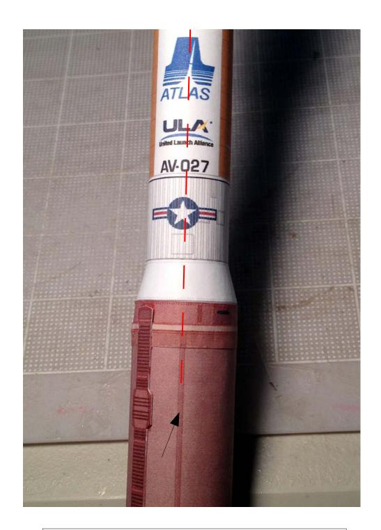
If aligned properly, then all the upper logos and flag should align with the 2 thin lines shown with the arrow.
